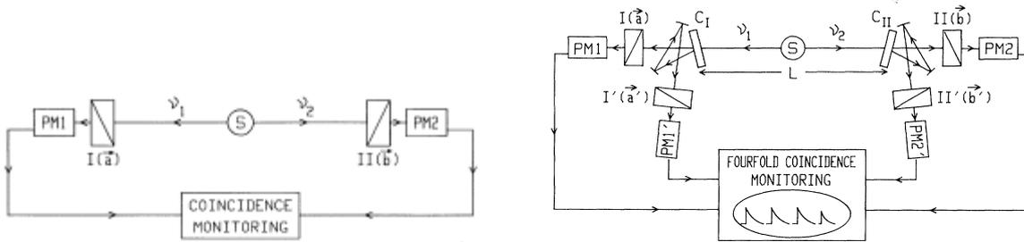
Figure 2: *Left* Optical version of an EPR experiment, the pair of photons  $\nu_1$  and  $\nu_2$  is analysed by linear polarisers I and II. *Right* Timing experiment with optical switches, each switching device is followed by two polarisers in two different orientations (Figures taken from Ref.[11]).
